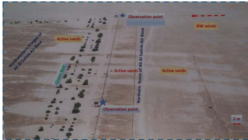
Figure 31.16. Low altitude aerial photograph showing the northwestern fringes of Ali Al Salem Air Base, note the existing green belt and the tongues of active sands (wind tunneling through gaps in the green belt).
