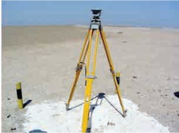
Plate 1. Base GPS unit positioned at a benchmark point
