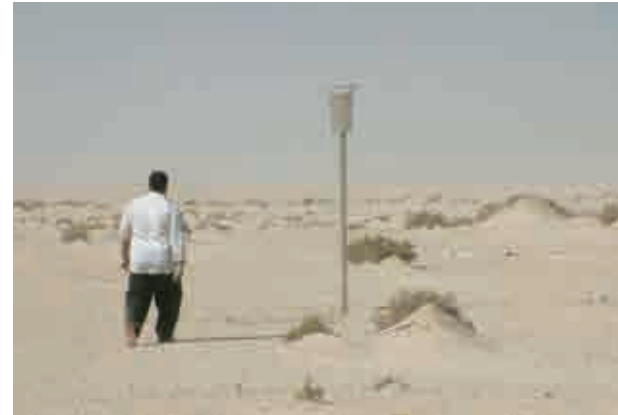
Plate 2. Dust collector (DC-10) installed in the southern part of Boubyan Island
