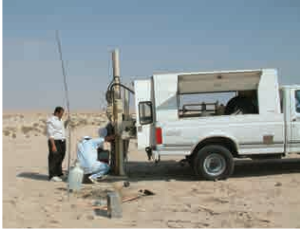
Plate 1. Drilling a piezometer 2 cm in diameter to 5 m deep by using a Geoprobe
