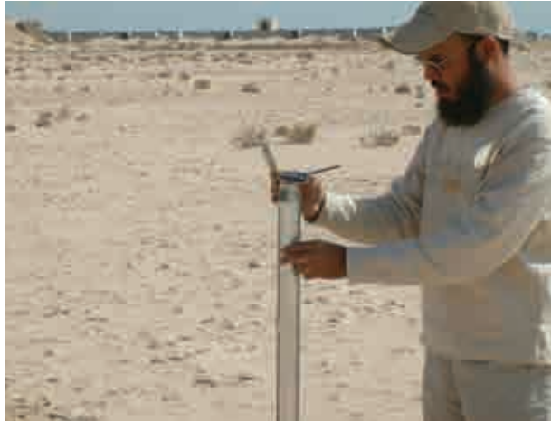
Plate 3. Leveling and directing the sand traps using a Brunton compass
